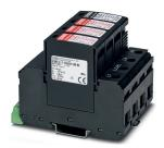
Surge protective device, four channel with remote indicator contact for 120/208 V Wye three phase AC, 4-wire plus ground.
