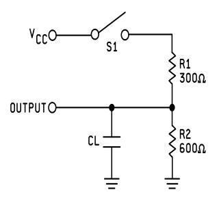
FIGURE 3. Switching test circuit.
