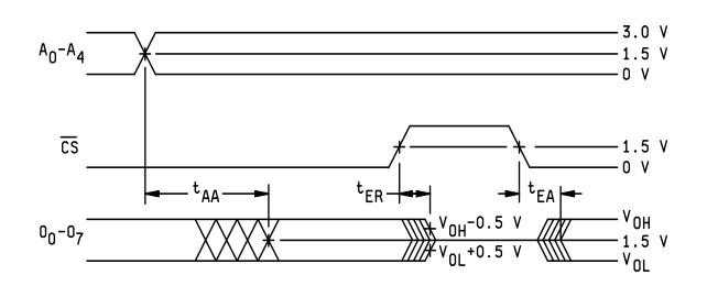
FIGURE 4. Switching waveforms.
