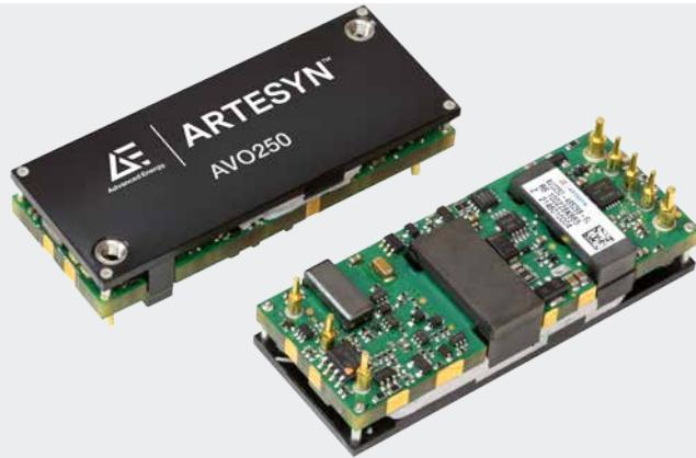
Advanced Energy's Artesyn AVO250 series eighth-brick isolated DC-DC converter provides a single regulated low noise 28 Vdc output. The converter has a wide 2:1 input range of 36 to 75 Vdc and is designed primarily for use with standard 48 V telecommunications equipment supplies. Rated at 250 watts, it can deliver up to 9 amps and accommodates an ambient operating temperature range of -40 to 85°C.
