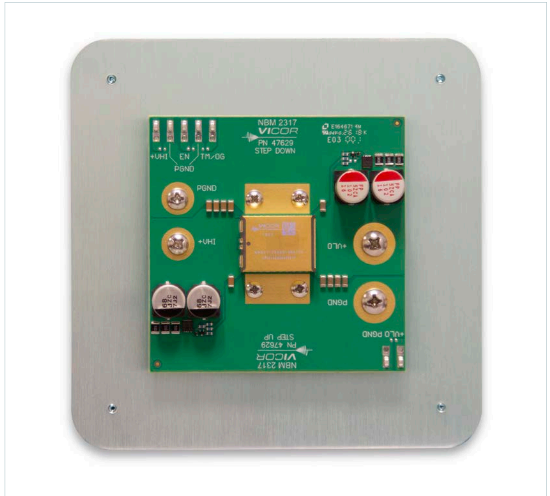
Figure 6 NBM™ evaluation board mounted on coldplate
