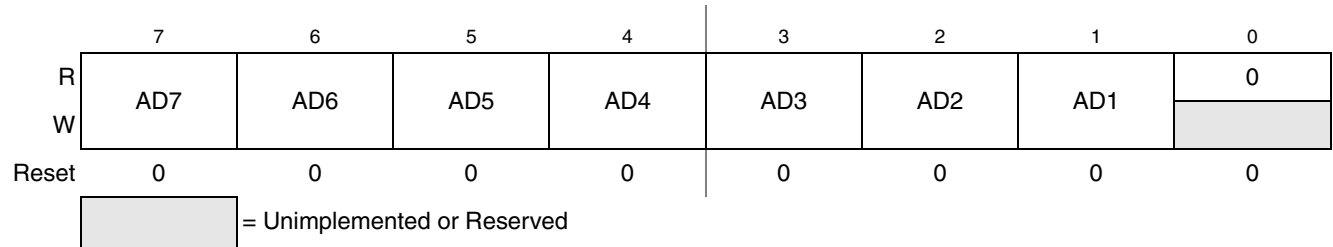
Figure 13-3. IIC Address Register (IIC1A)
