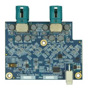
Since many different types of GMSL cameras are available, the JCB002 has user selectable options to interface with either GMSL1 or GMSL2 protocols at different operating frequencies.
