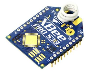
Xbee Pro RF Modules 928MHz 200Kbps 20-Pin w& Cortex-M3 EFM32G230 @28MHz - XBP9B-DMWT-022
