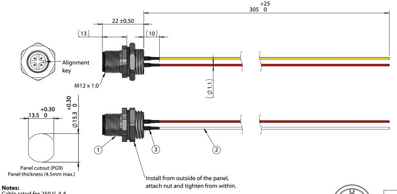
Cable rated for 250 V, 4 A Temperature:  $-40 \sim 105$  °C
