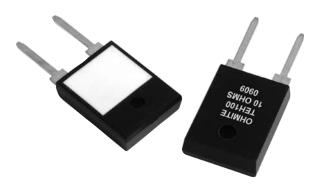
Ohmite offers the totally encapsulated and insulated TO-247 package for low ohmic value and non-inductive design for high-frequencv and pulsing applications. Ideal use is for power supplies. This series is rated at 100 Watts mounted to a heat sink.
