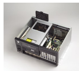
Solid disk drive housing & easy-to-maintain fan filter
