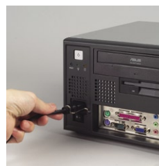
Power cord brace for fixing the power cord well
