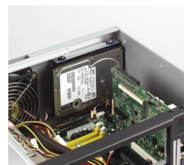
Shock-resistant drive bay for holding a 3.5" HDD
