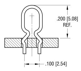
SHOWN AS **INSTALLED INTO** TWO .040 [1.02] DIA. **MOUNTING HOLE**
