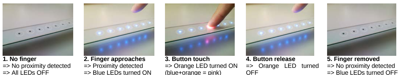
Figure 63 Touch+Proximity Module Operation
