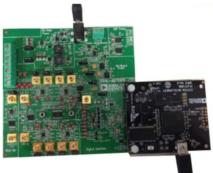
Figure 2. Evaluation Board (Left) Connected to the SDP Board (Right)
