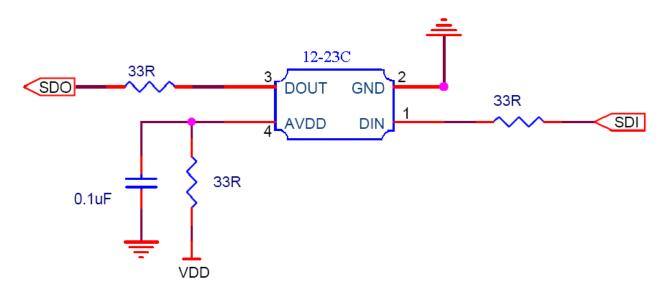
When 12-23C is set to operate on 5V power system, a 0.1uF capacitor is recommended to add between power supply and ground terminal. The capacitor is suggested to put as closer as possible to IC position. There are frequent resistors were used on different drain voltage as listed table.
