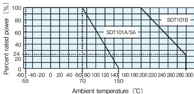
For sensors operated at an ambient temperature or higher, the power shall be derated in accordance with the above derating curve.
