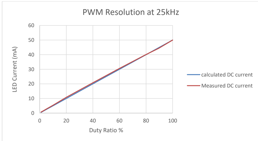
Figure 8 PWM Resolution with Power Path Switching (Refer to Figure 3c)
