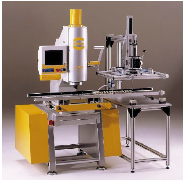
Fig. 8: Bestseller CPM prestige with insertion removal station, adaptable to all HARTING press-in machines.
