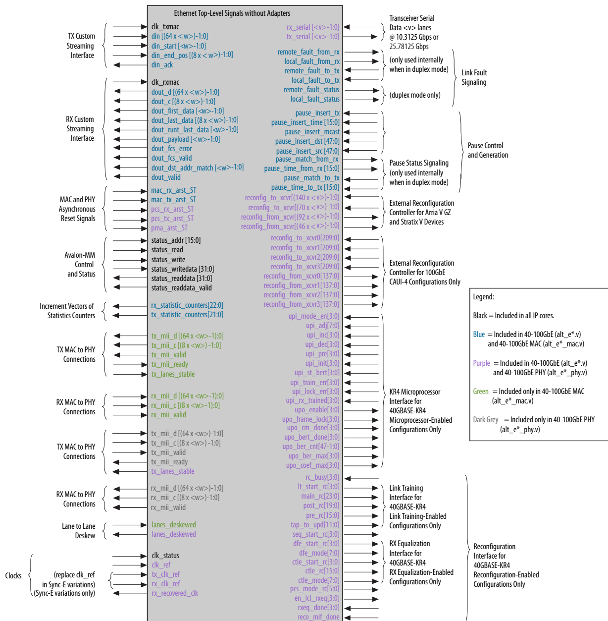
Figure 3-36: Top-Level Signals of the 40-100GbE IP Core Without Adapters
