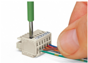
Inserting conductor via (2.5 x 0.4) mm screwdriver – CAGE CLAMP® actuation perpendicular to conductor entry.
