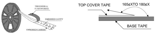
The force for peeling of cover tape is 10 grams in the arrow direction.
