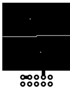
a. 93 ^\circ\text{C}/\text{W} when mounted on a 1 in 2 pad of 2 oz copper.
