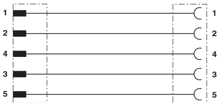
Contact assignment of the M12 plug and the M16 socket
