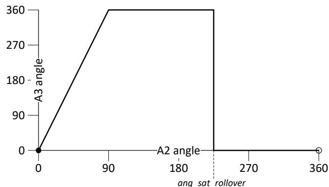
Figure 9: Angle gain behavior over full rotation with gain = 4 and output clamping enabled
