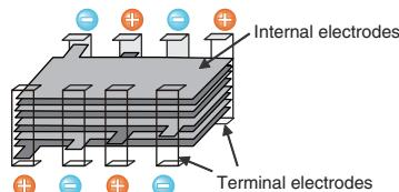
The eight terminal electrodes are connected +/- alternately to reverse the current flow and offset the magnetic field generated.
