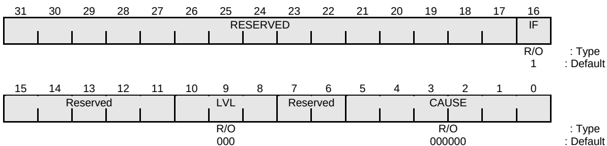
Figure 8-15 Interrupt Current Status Register
