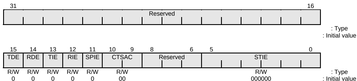
Figure 19-7 DMA/Interrupt Control Register
