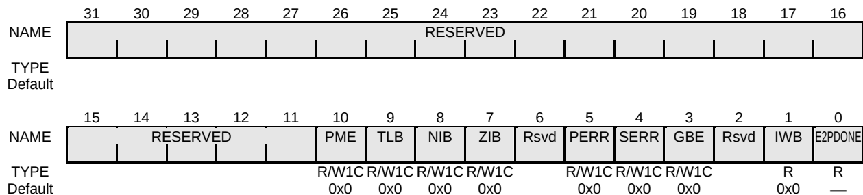
Figure 16-54 PCI Controller Status Register
