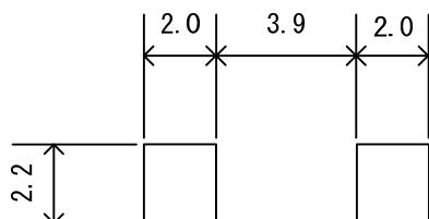
Adjacent land patterns and lines on the PCB should be covered with resist.
