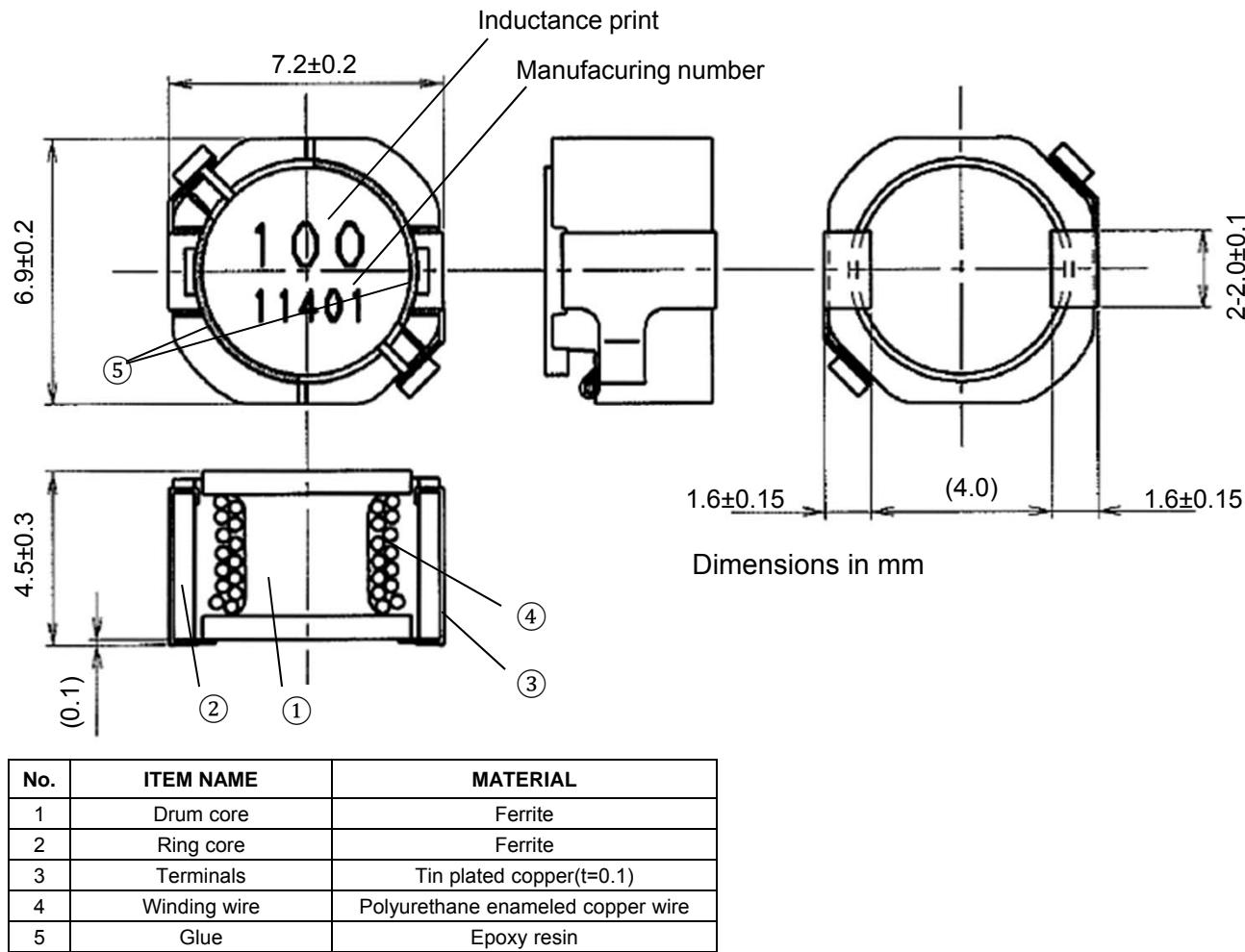
Note: 1) Even if the adhesives of an upper surface application have the portion which has not been buried completely, they presuppose that it is possible.
