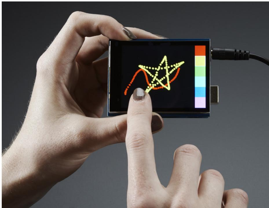
We now have a super-fancy capacitive touch screen version of this shield. Instead of a resistive controller that needs calibration and pressing down, the capacitive has a hard glass cover and can be used with a gentle fingertip. It is a single-touch capacitive screen only!
