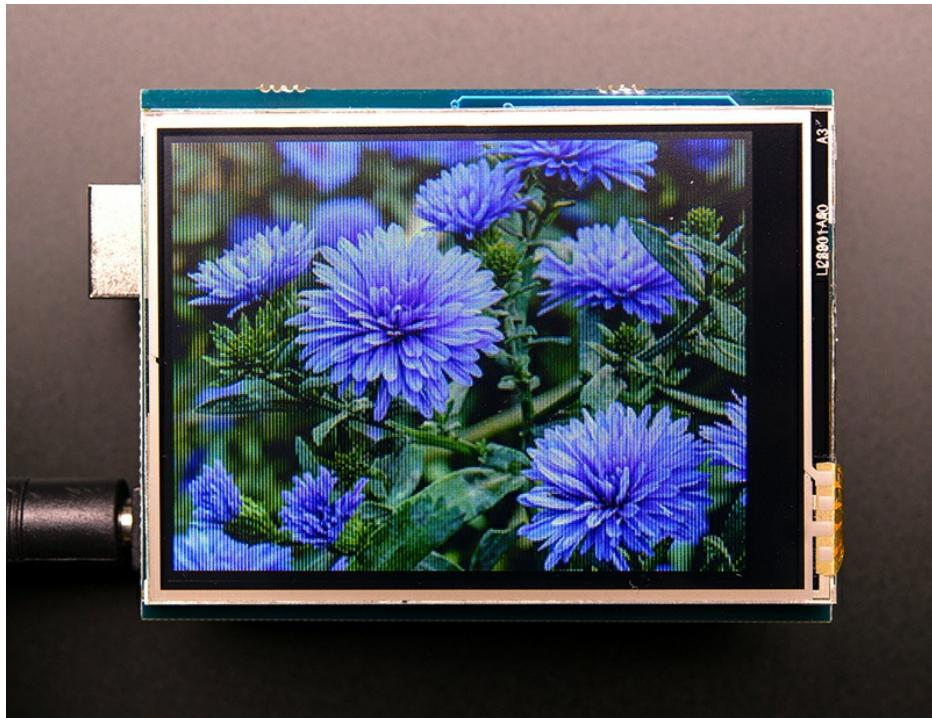
To make new bitmaps, make sure they are less than 240 by 320 pixels and save them in **24-bit BMP format!** They must be in 24-bit format, even if they are not 24-bit color as that is the easiest format for the Arduino to decode. You can rotate images using the **setRotation()** procedure.
