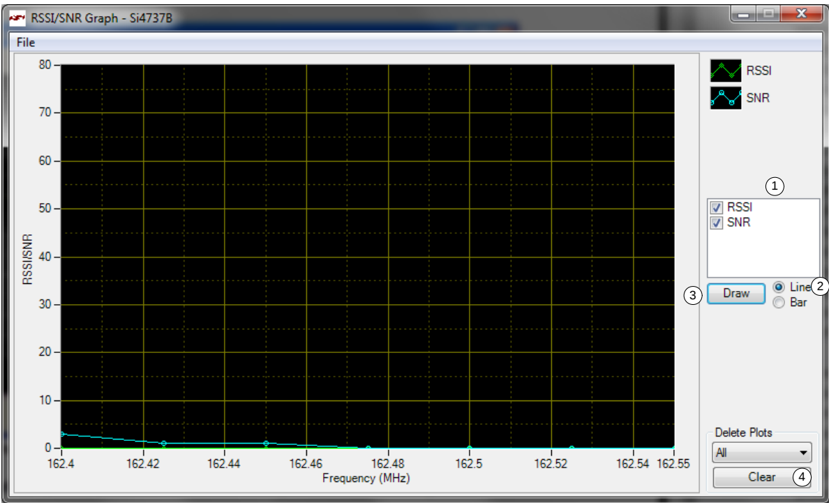
Figure 74. Weather Band Receiver RSSI/SNR Graph Window
