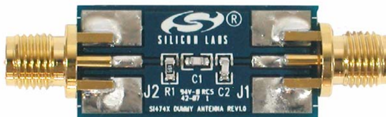
Figure 18. Si474x Antenna Dummy Card
