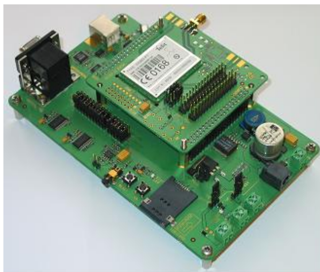
GE863-PY Interface Board (upper) fitted on EVK2 Motherboard (lower).
