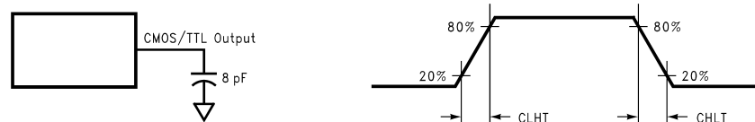
Figure 4. Receiver CMOS/TTL Output Load and Transition Times
