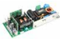
EVL011A150ADP 12 V - 150 W power supply based on TM PFC and HB LLC digital combo controller
