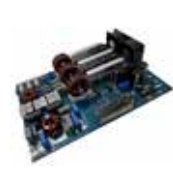
STDES-30KWVRECT 30 kW Vienna PFC rectifier reference design with digital control
