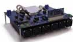
STDES-DABBIDIR 25 kW dual active Bridge (DAB) bidirectional power converter for BESS and EV charging
