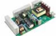
EVL400W-80PL 12 V - 400 W adapter based on CCM PFC and HB LLC analog controller
