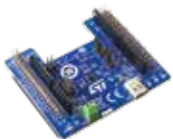
X-NUCLEO-SRC1M1 USB Type-C power delivery source expansion board based on TCPP02-M18
