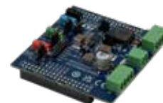
STEVAL-SPSA068 PMIC evaluation board based on SPSA068
