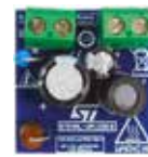
STEVAL-VP12201B 15 V/200 mA buck converter
