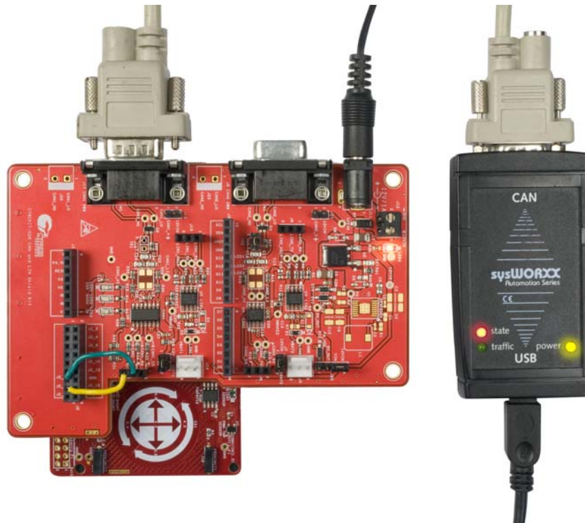
Figure 4-2. CAN Analyzer Connection to CY8CKIT-026's CAN1 Transceiver
