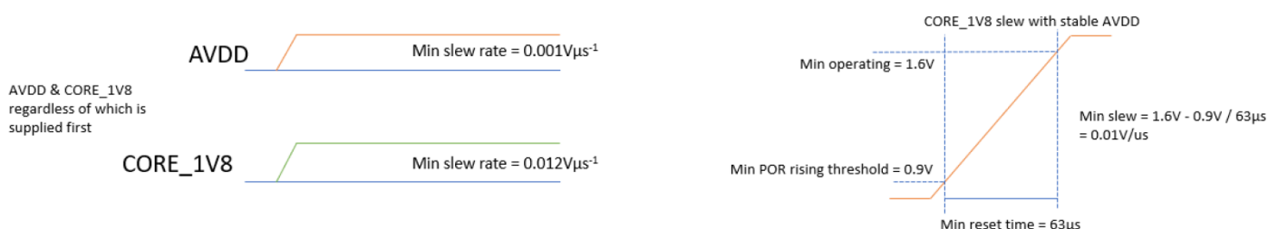
Figure 9. Power up slew
