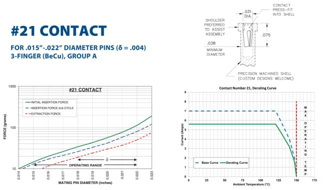
The insertion / extraction force characteristics above were derived using a 30 microinch gold-plated contact and polished steel gauge pins having a bullet-shaped tip. The curves represent typical average values; they are best used to compare the differences between similar size contacts and to guide you in selecting one that is suitable for your application. Your results may vary, so for your specification, we encourage you to obtain complimentary samples for your evaluation.
