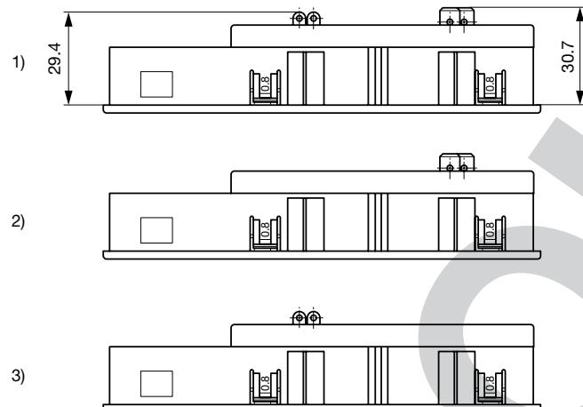
1) Solder and quick connect terminals 6.3x0.8 mm
