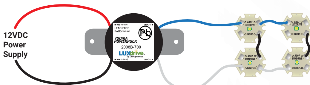
PowerPuck 2008B-700 driving (4) Cree™ or Luxeon™ LEDs from 12VDC.
