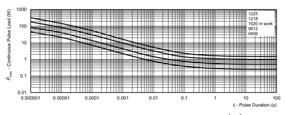
Maximum pulse load, continuous pulses; applicable if  $\overline{P} \leq P(v_{amb})$  and  $U \leq U_{max}$ ; for permissible resistance change equivalent to 8000 h operation
