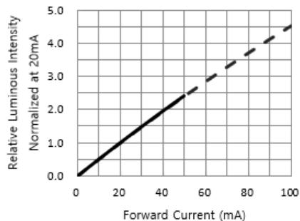
**Fig. 4 RELATIVE LUMINOUS INTENSITY VS. FORWARD CURRENT**
