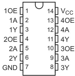
**Figure 3-1. SN74LVC126A-Q1 D or PW Package;
