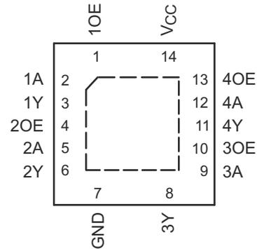
**Figure 3-2. SN74LVC126A-Q1 BQA Package; 14-Pin
