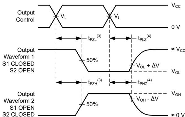
(1) The greater between t<sub>PZL</sub> and t<sub>PZH</sub> is the same as t<sub>en</sub>.
