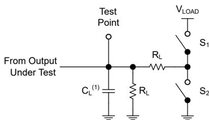
(1) C<sub>L</sub> includes probe and test-fixture capacitance.
