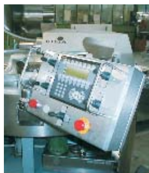
Example 16 Premium Panel with side support arm connection CP-S. Particularly suitable for use in the food industry
