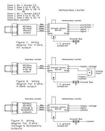
The transducers listed below are designed for installation in EITHER Class I, Division 1, Groups C,D; Class I, Zone 0 Group IIB DR Class I, Division 1, Groups A,B,C,D; Class I, Zone 0 Group IIC hazardous locations when connected to Associated Apparatus as described in note 1.
