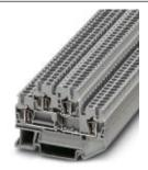
Component terminal block, with integrated diode 1N 5408K, Connection method: Spring-cage connection, Cross section: 0.08 mm² - 4 mm², AWG: 28 - 12, Nominal current: 1.5 A, Nominal voltage: 500 V, Length: 67.5 mm, Width: 5.2 mm, Color: gray, Assembly: NS 35/7,5, NS 35/15
