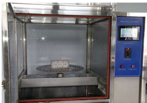
Testing under water jet
