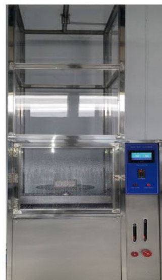
Testing under water jet
