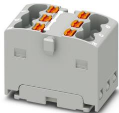
Distribution block, Basic terminal block, nom. voltage: 450 V, nominal current: 17.5 A, number of connections: 6, connection method: Push-in connection, cross section: 0.14 mm<sup>2</sup> - 2.5 mm<sup>2</sup>, mounting type: adhesive, color: gray
