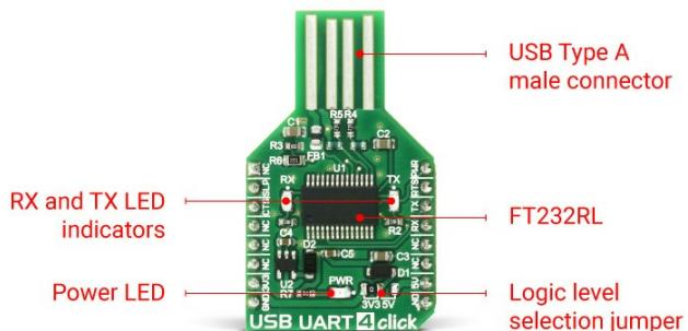
This device also features the configurable CBUS pins, which can be used for several different useful functions, as for example - configurable clock out for driving the microcontroller, data LED drive, USB Sleep, PWR status and so on. By default, CBUS3 and CBUS4 pins are configured as Power Enable and Sleep options and are routed to the PWR and SLP pins of the mikroBUS™. More information about configuring the CBUS pins can be found in the [FT232RL datasheet](#).
