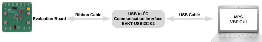
Figure 1: Evaluation Kit Set-Up
