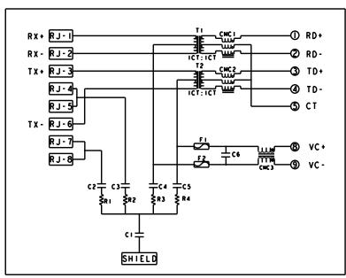
CI = 1000pF, 2KV, ±10%, X7R DECOUPLING CAP C2 - C5 = 22nF, 100V, ±10% CAPACITORS RI-R4 = 75 Ohms, 1/16 W, ±5% RESISTORS C6 = 0.1uF, 100V FI-F2=125V, IA
