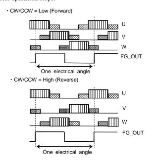
2) Output of rotation speed signal: FG\_OUT pin
