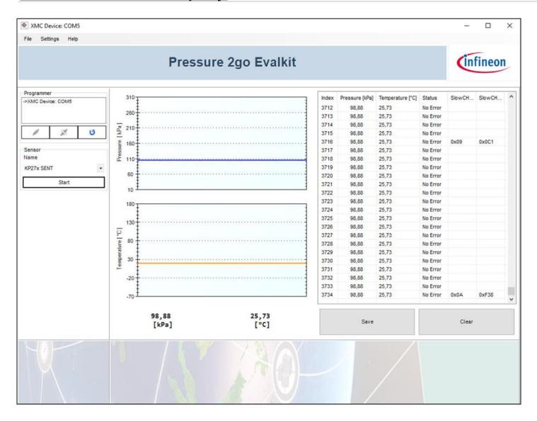
Real time graph for plotting pressure and temperature value.
