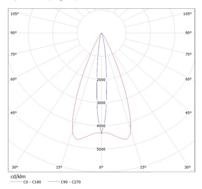
Luminaire: Ledil Oy CA12589\_EMILY-WWW (Cree XP-G 58Im @ 250mA) Efficiency=86% Lamps: 1 x Cree XP-G 58Im @ 250mA
