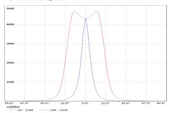
Luminaire: Ledil Oy CA12589\_EMILY-WWW (Cree XP-G 58Im @ 250mA) Efficiency=86% Lamps: 1 x Cree XP-G 58Im @ 250mA
